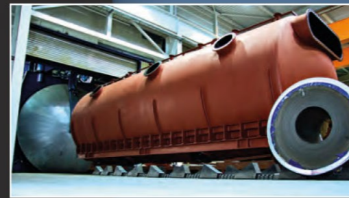
Rubber linings workshop: The best possible rubber lining quality is achieved in Steuler autoclaves at high temperatures and pressures.
